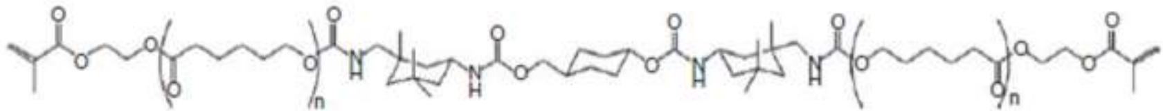
Structure of a Monomer with Cycloaliphatic Units
