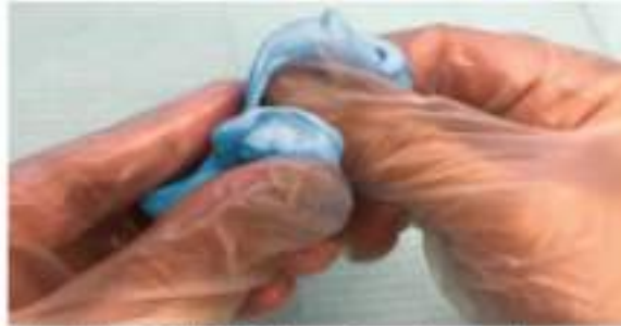
Knead the FLEXCEED base & catalyst until a uniform blue color is achieved.
